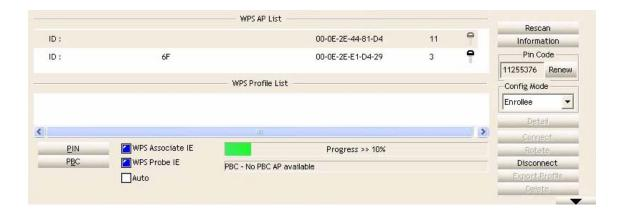
**Step 1.** Click on 'PIN' button now, and wait for few seconds to one minute. If a wireless access point with correct PIN code is found, it will be connected to that device.
